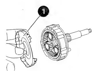
Checking planetary gear train
